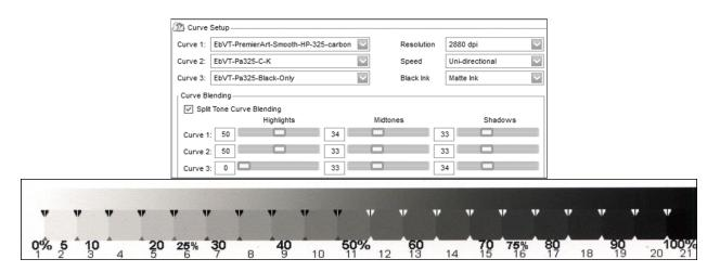
For large wall prints, it is doubtful that anyone will notice the slight graininess of this print. This test strip original was 8 inches wide. The image is 200 dpi. The Lab B of the paper was adjusted to Lab B = 0 so that the "brighter" background of the Word document would not bias the delta B = 2.6 of the print as it would be seen displayed on the wall (and not around bright paper or monitors). The colors of the scan are not particularly accurate.
