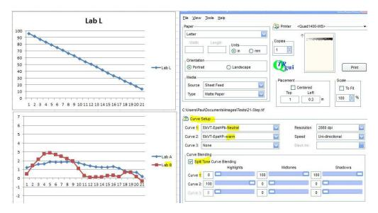
A more common use of the QTR sliders is simply to combine a carbon/warm with a neutral profile to achieve a print tone that is between the two. Thus with the 100% carbon and toned "neutral" profiles, all the intermediate print tones are available.
