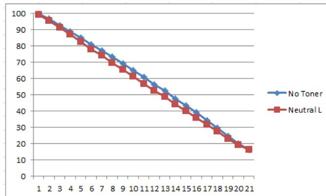
As can be seen in the above graphs, the additional density added by the toner is never as much as the 5% difference between the steps of the 21-step test strip. If the color pigments totally disappeared, aside from a side-by-side comparison, viewers would not notice a density difference.
