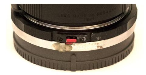
The (red) "key" (my term) on the VM-E focusing ring is easy to remove and file so that its edge is at the appropriate place relative to the keyhole in the stationary part of the VM-E mount. To shorten the keyhole at the other side, a small (just under 3 mm) piece of metal was cut off some metal plumbers
