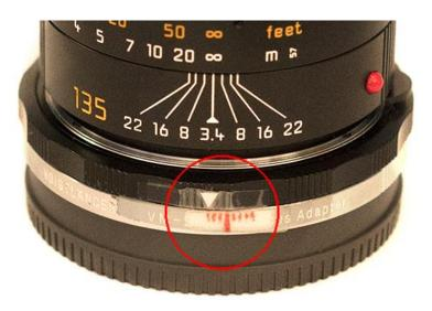
There is a strip of white label paper with red marks that are 1 mm apart. This is attached and taped to the stationary part of the mount. On the mount's focusing ring I tape a triangular marker. With the VM-E mount focused all the way in, the marker is at the first of the 1 mm red marks.
