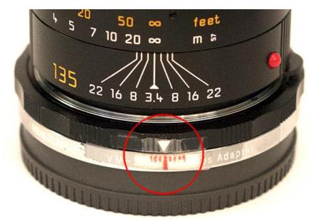
It is best to be able to lock the VM-E focus ring at this point. One could use tape to do this. An easier to lock and un-lock system would be helpful.
