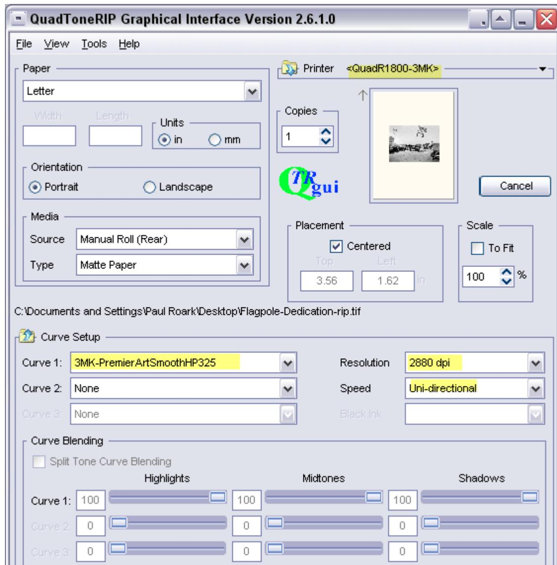
The 3-MK workflow makes quite neutral prints on un-brightened, “natural” (no OBAs) papers. It has a very fine grained image structure that also tends to impart a sense of finer detail than is actually in, for example, an old photo reproduction. Eboni carbon on un-brightened paper is probably the most stable print. Epson’s “most archival” (and relative bargain) Premier Matte Scrapbook cotton paper and 100% Eboni carbon pigments may make the most stable image.
