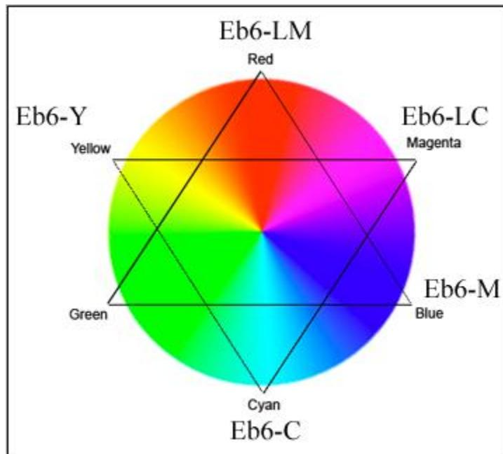
By being in the order of the color wheel, RGB curves, embedded in B&W ICCs, can be made to start the inks in their density order.
