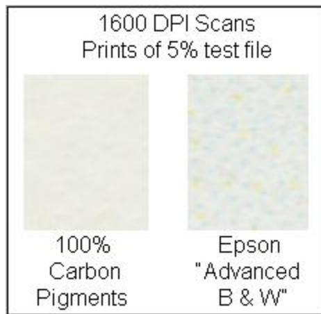
With no color pigments and many more carbon channels and levels, the 100% Carbon pigment Eboni-1800 prints have a significantly different image structure than the Epson “Advanced Black and White” mode prints. See the high resolution (1600 DPI Epson flatbed) scans of prints made with the 2 different approaches. When the dilute Eboni-6 inks are used, the image is exceptionally smooth, as seen above.
